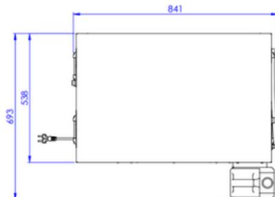
Our chillers feature a double-circuit insulated enclosure that accumulates high levels of refrigeration through the formation of ice in the tank water.
